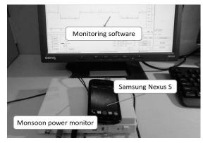
Fig. 6: Energy consumption experimental setting.
