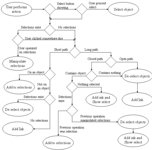
Figure 2: The decision tree used to reason about user input with the inferred mode protocol.
