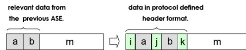
Fig. 1.6. An abstract representation of recasting data from a previous ASE into the protocol defined header format.
