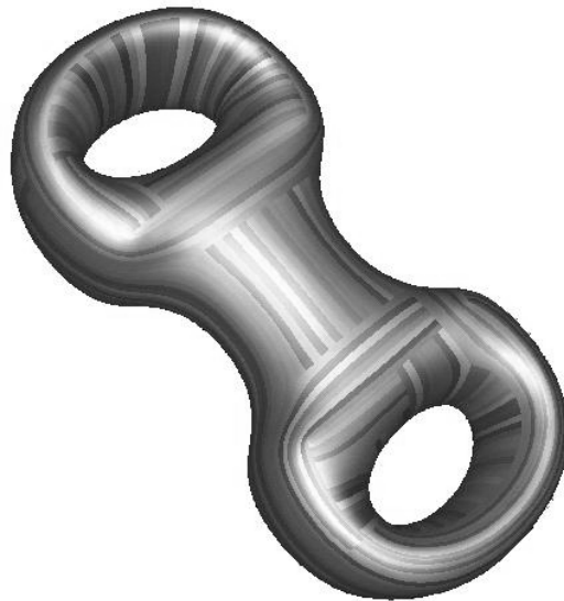
Figure 3.3: A genus two object subdivided using longitudinal strips
