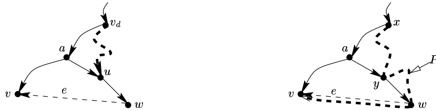
Figure 5: Computation of \text{detour}(e) for a cross edge. The case of a back edge is similar.
