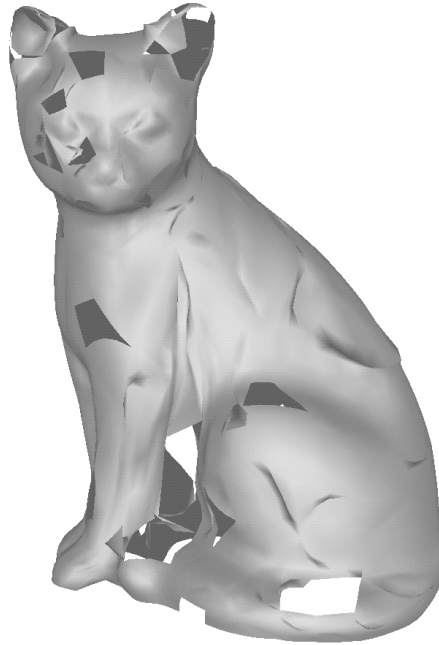
Figure 5.4: Parametric Foley-Opitz patches fitted to the cat data set using a projection plane that is perpendicular to the bisecting plane. Patches failing to meet the tolerance C_i = 3 and C_b = 3 were not rendered. 76 of 698 patches failed to meet the tolerance conditions.
