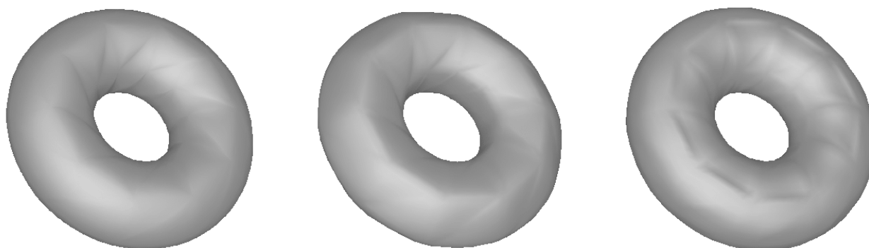
Figure 5.11: Comparison of Shirman-Sequin, triangular Gregory patches, and parametric Foley-Opitz patches on the 10 x 5 torus data set using planar boundary curves with Shirman-Sequin and triangular Gregory patches.
