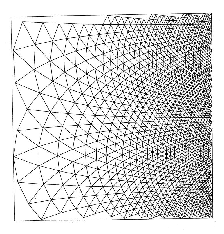
Fig. 10. Optimally efficient triangulation for Example 1
