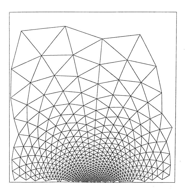
Fig. 15. Optimally efficient triangulation for Example 2
