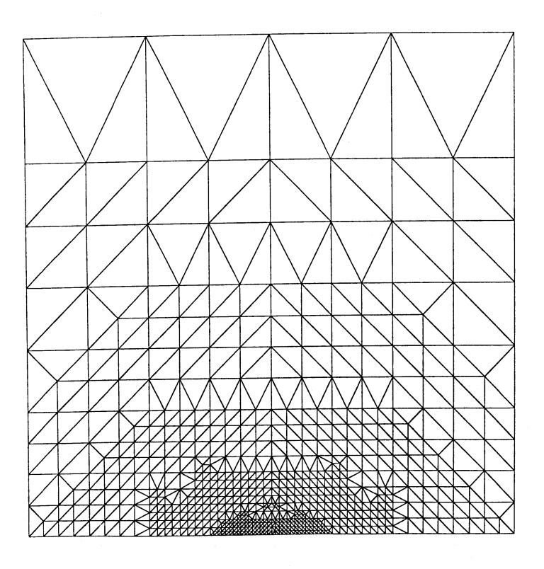
Fig. 14. Mesh produced by PLTMG for Example 2
