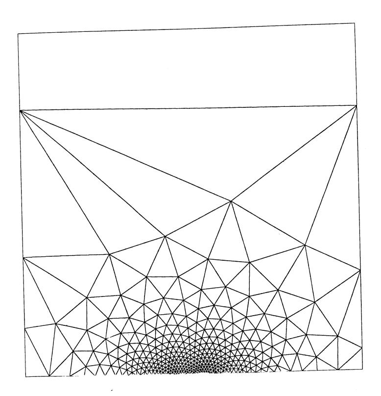
Fig. 18. Mesh produced by equilateral triangles for Example 3
