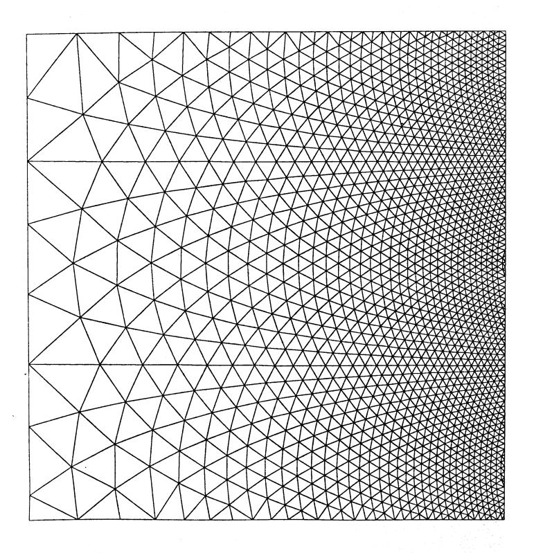
Fig. 8. Mesh produced by equilateral triangles for Example 1
