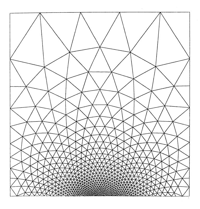
Fig. 13. Mesh produced by equilateral triangles for Example 2
