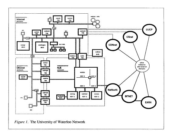
The IBM complex is connected to four of the VAXes using an RSCS network running NJE protocols, while the Honeywell computer is connected to a VAX using a synchronous HDLC link. The various Ethernet networks are joined together by LAN Bridge 100s, a network level bridge which can control the movement of traffic between networks.
