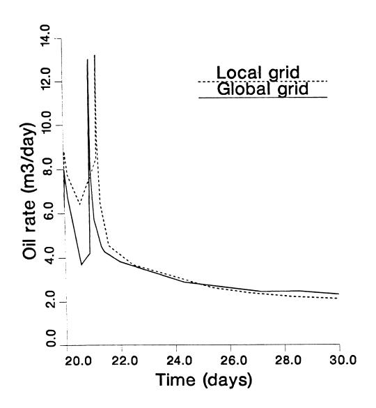
Comparison of oil rates for the locally refined grid and conventional global grid for the fracture problem.
