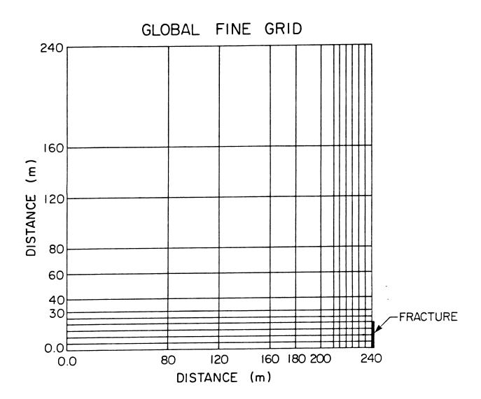
Typical global grid for simulation of an areal fracture problem.
