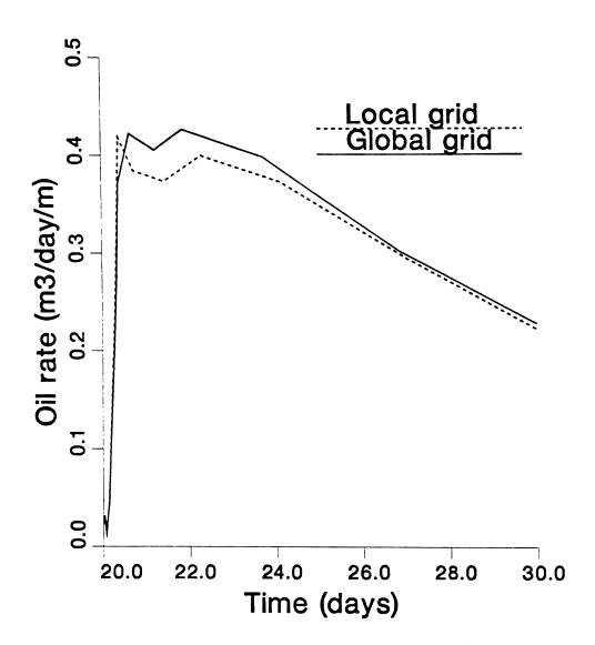
Comparison of oil rates for the locally refined and conventional global grid for the cyclic steam cross section.
