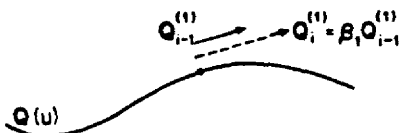
Figure 200. The basic idea behind the notion of G^1 continuity is that the tangent vectors at the joint between two successive segments need only be collinear; their magnitudes may differ by a positive factor which we are calling \beta_1 .
