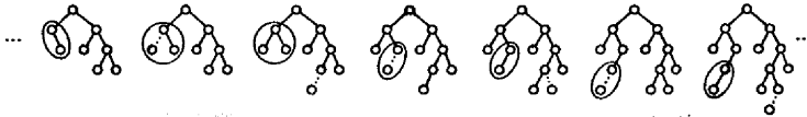
Fig. 7.2.2 Instances of the fringe of a binary search tree when random insertions are performed (fringe is encircled)
