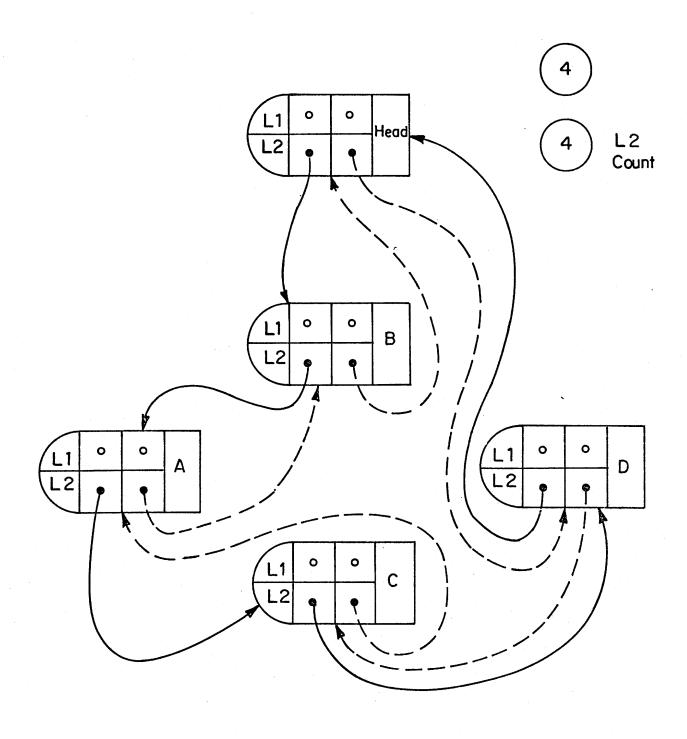
Fig. 4.1(b) Compound structure showing second list (L2) pointers. Logical order (B,A,C,D)
