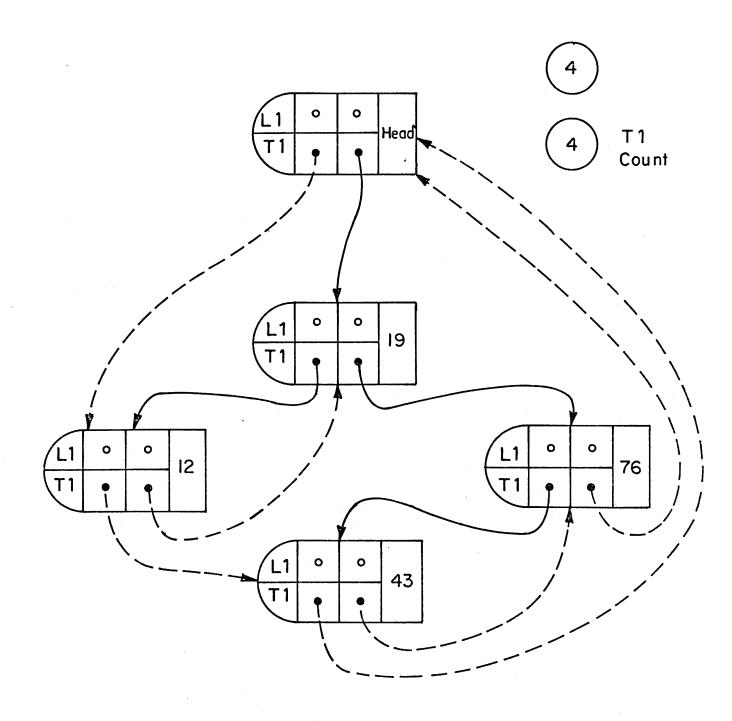
Fig. 4.2(a) Compound binary tree—linked list, showing tree pointers, threads and chains
