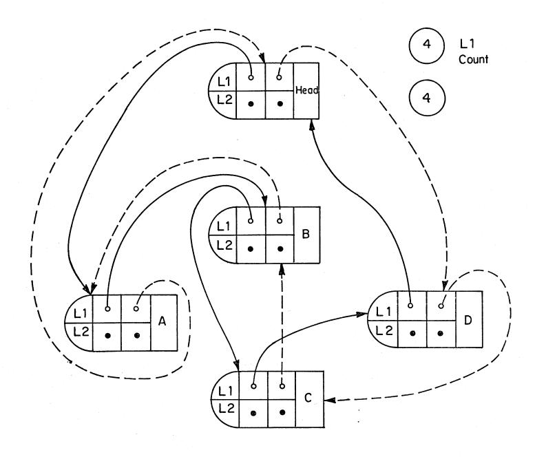
Fig. 4.1 (a) Compound structure showing first list (L1) pointers. Logical order (A,B,C,D)
