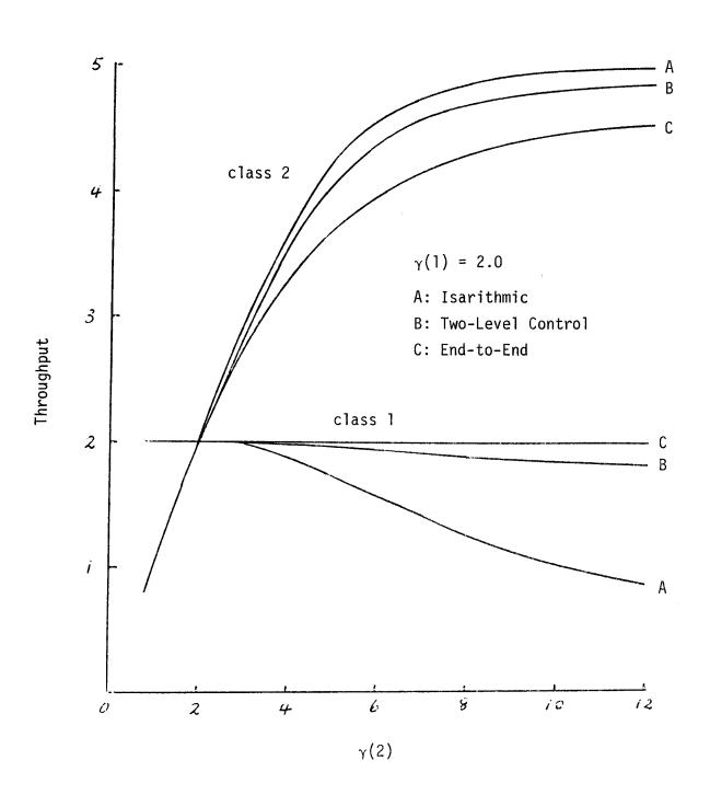
Figure 3 Tandem Link Model: Total Throughput vs.  $\gamma(2)$
