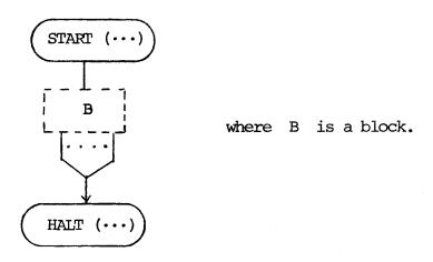
Clearly every flowchart in block form is equivalent to some program schema. The result of Engeler and Cooper is that for every program schema we can find an equivalent flowchart in block form.
