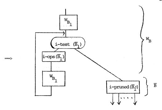
iii) B is the concatenation of  ${\rm B_1}$  and  ${\rm B_2}$  , using the i-th exit of  ${\rm B_1}$  :
