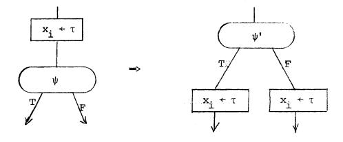
where  $\psi$ ' is like  $\psi$  but with  $x_i$  replaced by  $\tau$  . It is then a simple matter to find a single test to 'extract' the i-th path by repeatedly applying the transformations:
