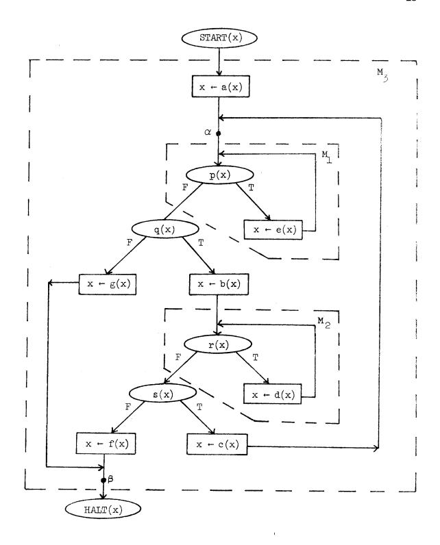
Figure 2. The module form flowchart  $P_1^n$  .
