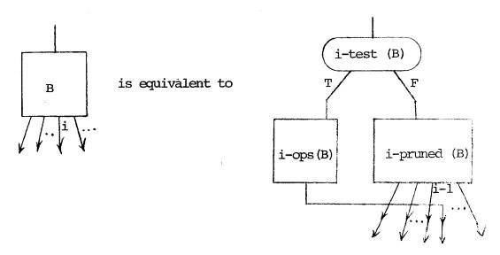
To see this, note first that the basic block can be put into a form in which the tests on the path to the i-th exit precede the assignments, by repeated application of the transformation:
