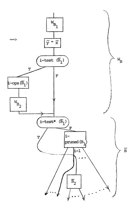
$\overline{x}$  is a vector of the variables occurring in i-test( $\overline{B}_1$ );  $\overline{y}$  is a vector of the same length of  $\underline{new}$  variables; i-test\*( $\overline{B}_1$ ) is the same as i-test( $\overline{B}_1$ ) but with variables  $\overline{x}$  replaced by  $\overline{y}$ , so that any computation must take the same branch out of each test.
