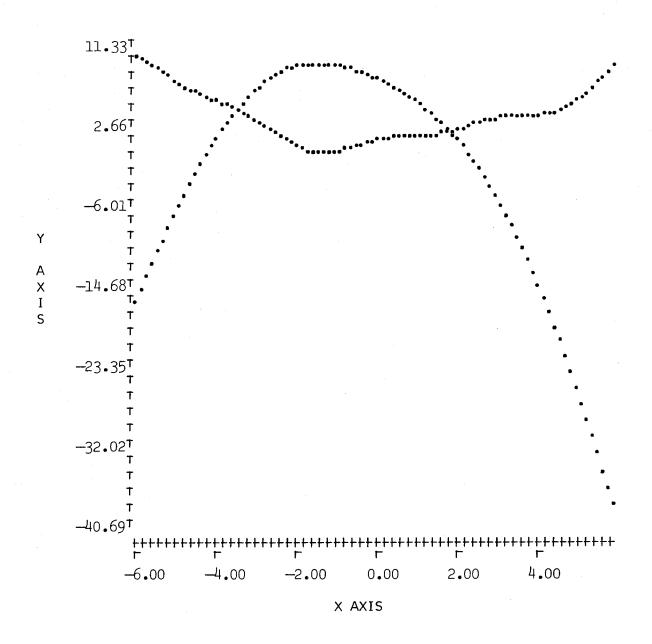
WHEN YOU USE THIS DEVICE, REMEMBER ALWAYS TO ENCLOSE YOUR ENTIRE FUNCTION IN EACH LINE WITHIN BRACKETS, JUST AS WE DID ABOVE, OTHERWISE YOU WILL GET GARBAGE OUT. THE INTERSECTION POINTS OF THESE TWO GRAPHS APPEAR TO BE AT ABOUT AN X VALUE OF -3.5 AND 1.8. BY REPLOTTING THE CURVE, WHICH WE WILL NOT DO, AND RESETTING THE LIMITS FOR X YOU COULD PLOT THESE POINTS EVEN MORE ACCURATELY.
