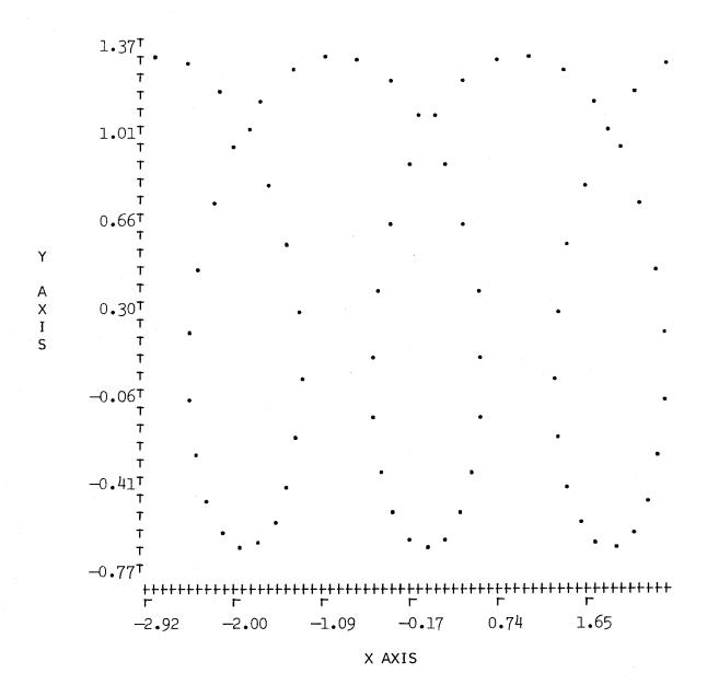
FINALLY, WE OBSERVE THAT THE SCALING ON THE Y-AXIS IS GROSSLY EXAGGERATED. TO MAKE THE X AND Y AXIS SCALING APPROXIMATELY EQUAL WE TURN OFF THE AUTOMATIC SCALING FOR THE Y-AXIS BY TYPING
