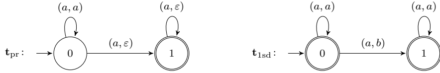
Figure 1: The left transducer is input-altering and describes the prefix codes: on input x it outputs any proper prefix of x . The right transducer is input-preserving and describes the 1-substitution error-detecting languages: on input x it outputs either x or any word differing from x in exactly one position.
