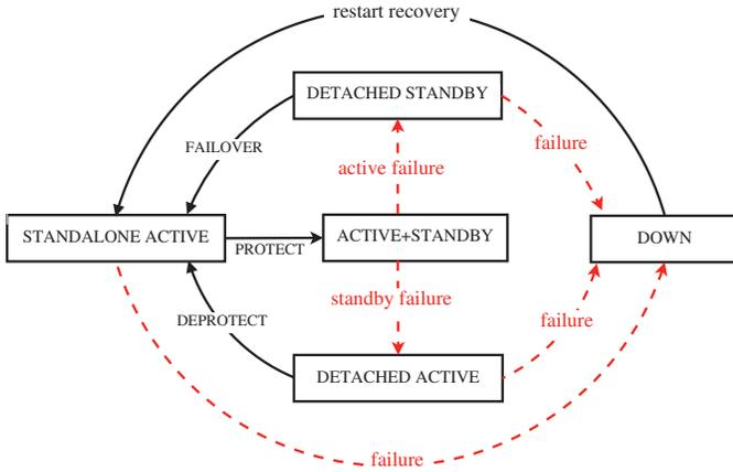
**Figure 3.** Operational States of a SHADOW System
