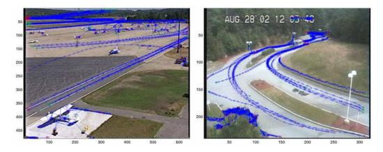
Figure 3: A composite of motion tracks detected by our system in two different settings: an airport tarmac (left), and an entrance gate to an office park (right).
