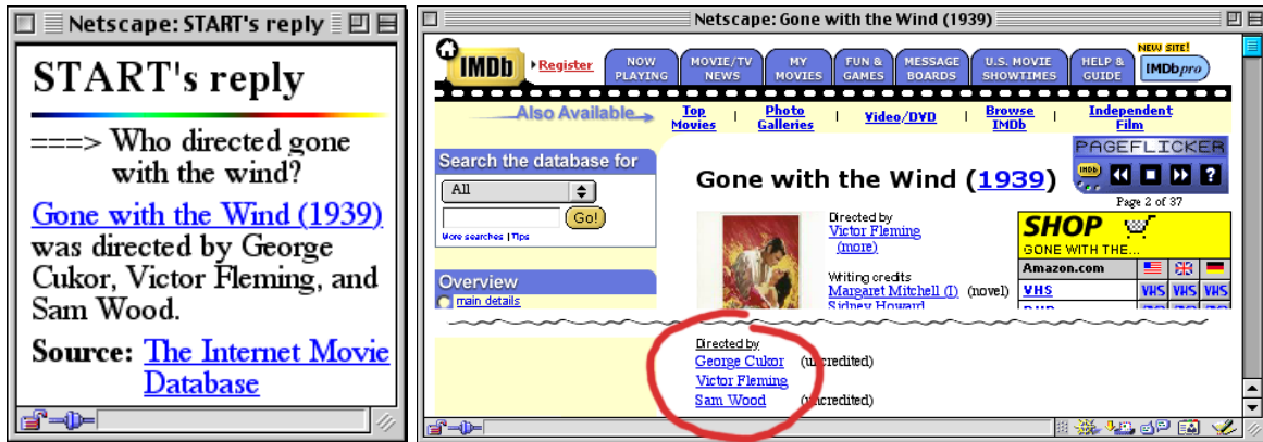
Figure 5: START’s response to “Who directed Gone with the Wind ” and the original Web page from which Omnibase extracts the answer.
