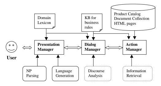
Figure 1: System Architecture
