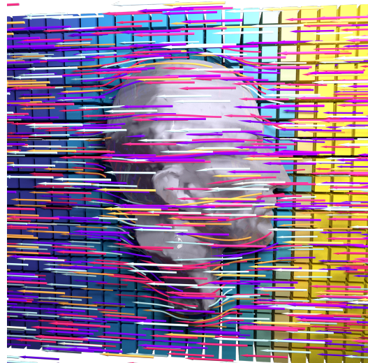
Fig. 22. We simulate the effect of putting a bust of Max Planck in a wind tunnel. In the background we show the resulting pressure field as per-cut-cell colors and in the foreground we show the resulting flow with arrows. Note how the arrows flow around the bust.
