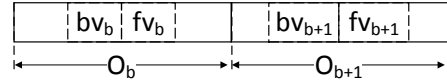
Figure 9: Joint versions for lock-free reads of adjacent buckets. The two objects are consistent with each other if they are individually consistent and fv_b = bv_{b+1} .
