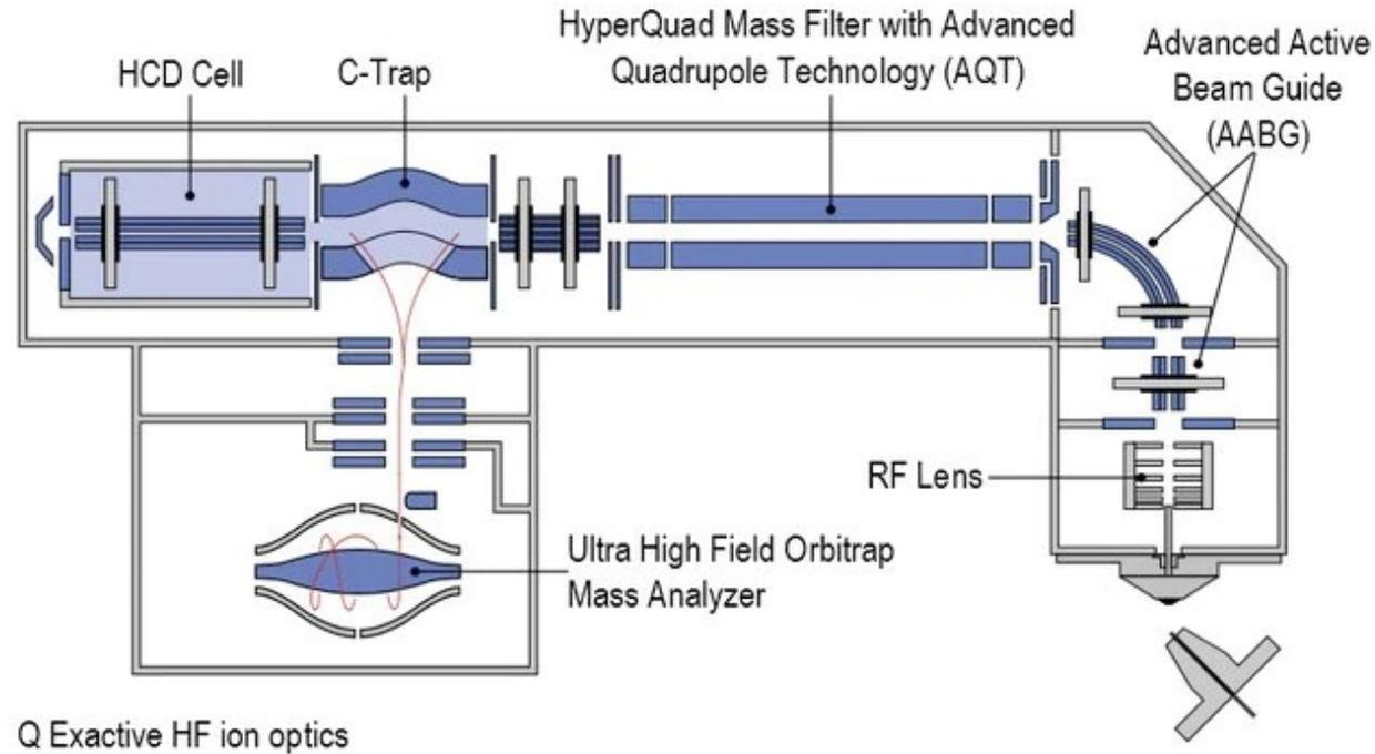
An actual instrument may consist many components for better sensitivity, accuracy, throughput and robustness. The figure illustrate the main components of an Orbitrap QE-HF instrument made by ThermoFisher Scientific.
