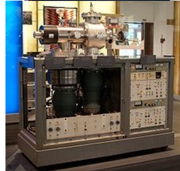
Fenn's first electrospray ionization source (top) coupled to a single quadrupole mass spectrometer
