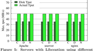
Figure 5: Servers with Libception using different block I/O schedulers
