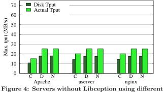
Figure 4: Servers without Libception using different block I/O schedulers
