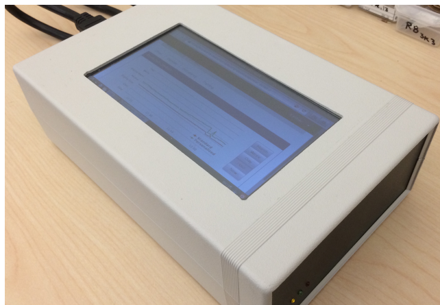
Figure 6: For isolated installations of SPOT*, a 7-inch touch screen LCD is mounted on the actuation box. This LCD is connected to the RPi inside the box and provides a local GUI to the user. In this configuration, which has the best privacy protection, occupancy data remains physically in the office.
