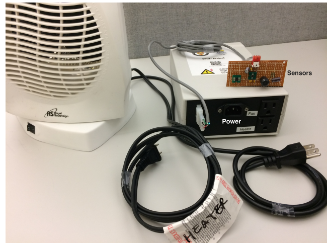
Figure 2: Hardware components of actuation and sensing in SPOT*. The fan/heater is shown on the right side, and the actuation box is on the left side. In this picture, the two independent power cords of the modified fan/heater are connected to the box. The modular design of the box, allows usage of different types of fans and heaters.
