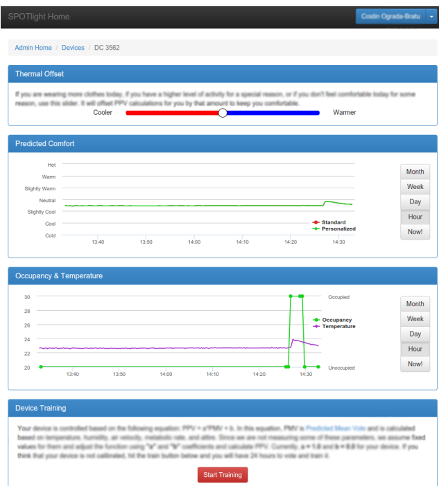
Figure 5: The graphical user interface, viewable with standard internet browsers. The top section allows users to manually fine-tune the system for temporary changes. The graphs in the middle visualize comfort (PMV and PPV), occupancy, and temperature over time. Users use the bottom section to start training their devices. During the training, users vote periodically on how they feel based on the 7-point ASHRAE scale.
