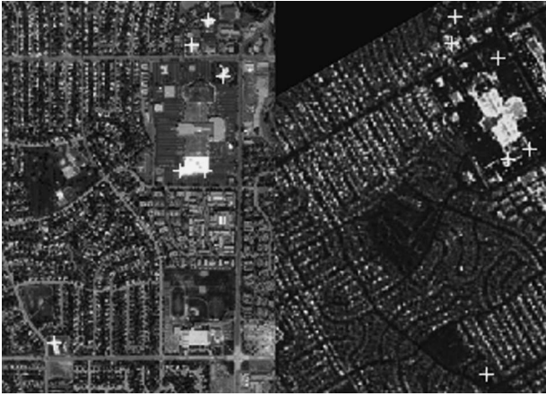
Fig. 2. Final set of candidate CPs (as indicated by crosses). (Left) Optical image. (Right) LIDAR image.
