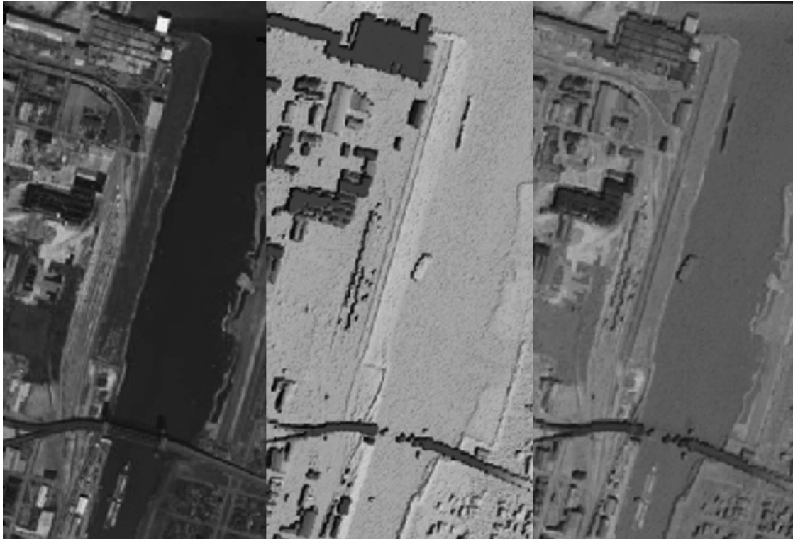
Fig. 5. Image registration from the TEST3 test set. (Left) Optical image. (Center) LIDAR image. (Right) Aligned images.
