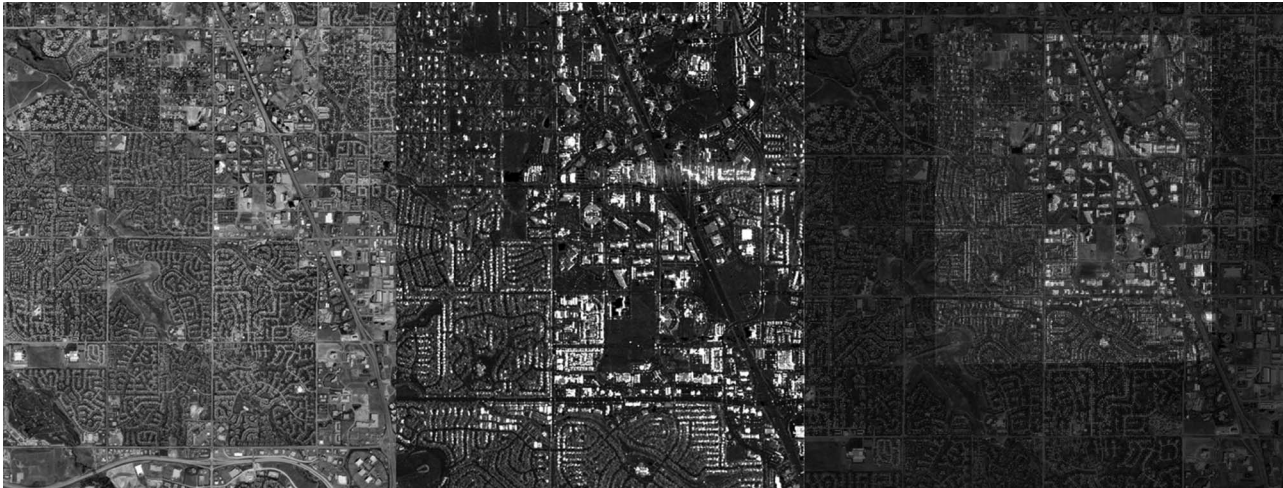
Fig. 3. Image registration from the TEST2 test set. (Left) Optical image. (Center) LIDAR image. (Right) Aligned images.
