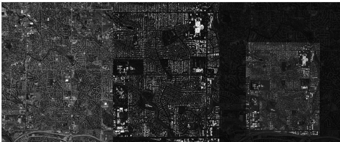
Fig. 4. Image registration from the TEST1 test set after rotation. (Left) Optical image. (Center) LIDAR image. (Right) Aligned images.
