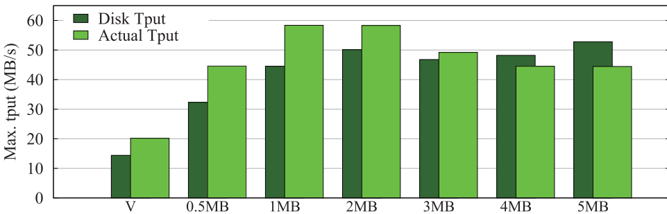
Fig. 15. nginx without Libception using various read_ahead_kb sizes, with max_sectors_kb = 16MB (Linux, WD drive).
