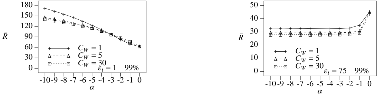
Figure 4: Mean response time vs. scheduling algorithm ( \alpha ); load=90%, jobs are not perfectly efficient
